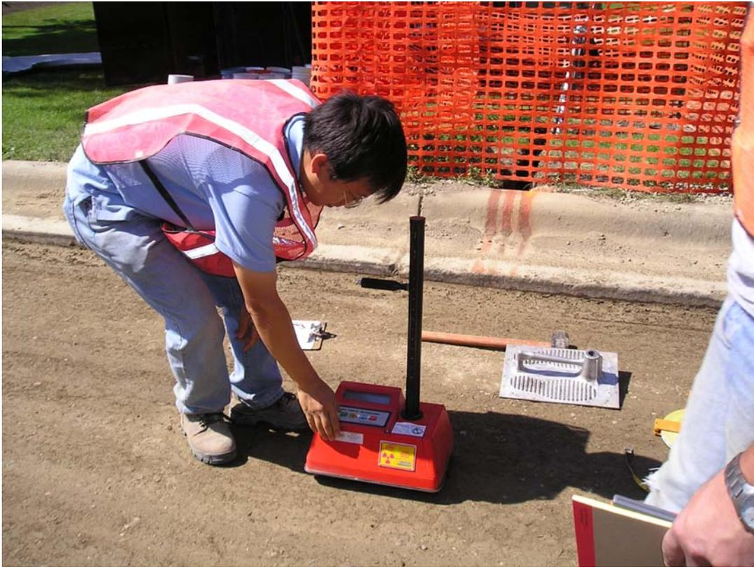
Fig. A8. Measuring water content and unit weight of SRPM after compaction.
